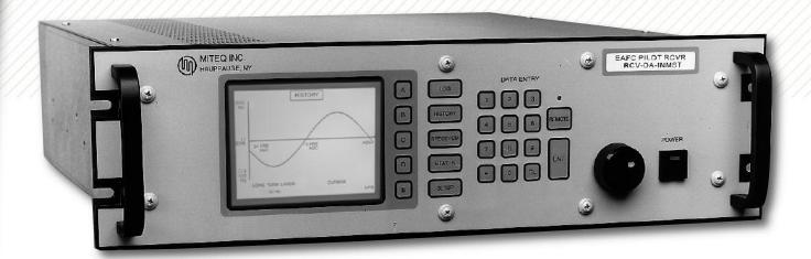
This receiver makes use of digital signal processing techniques to track a CW pilot signal. A phase continuous, 1 Hz step size, frequency synthesizer generates an error correction signal which is used in conjunction with MITEQ's INMARSAT AFC capable frequency converters to provide Automatic Frequency Control for both maritime and aeronautical (Enhanced AFC) applications.
