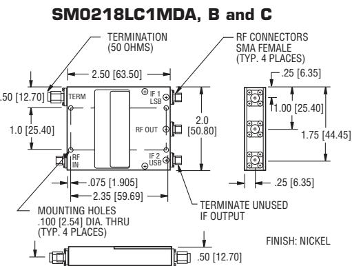
NOTE: All dimensions shown in brackets [ ] are in millimeters.
