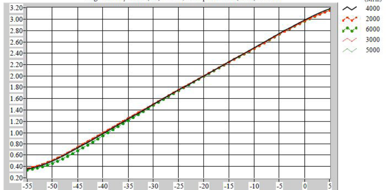
Video Output (V) Y Axis, Vs Input Power (dBm) X Axis
