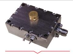
The L3Harris LCDRO is a free running DRO that is used in many microwave radar and radio frequency applications for both commercial and military.
