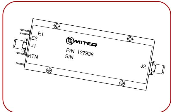
MITEQ's model 127938 integrated, two part, switchable filter bank features two channelized, printed circuit filter banks, individually selectable by TTL driven, SP2T PIN switches the input and output. MITEQ's Microwave Assemblies, Systems and Technologies Group specializes in the manufacture of integrated switch filter assemblies and is able to offer a wide range of frequency ranges and a number of channels.
