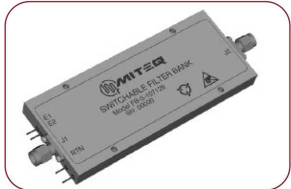
MITEQ's Model FB-S-107128 integrated, two part, switchable filter bank features two channelized, printed circuit filter banks, individually selectable by TTL driven, SP2T PIN switches the input and output. MITEQ's Microwave Control Products Group specializes in the manufacture of integrated switch filter assemblies and is able to offer a wide range of frequency ranges and a number of channels.
