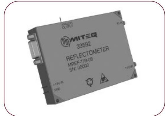
MITEQ's Model MREF-T/R-08 is an integrated assembly that contains a signal generator, transmitter, receiver and control circuitry. This unit transmits an RF signal, measures the reflected signal and then generates both an analog voltage and digital output that follows the level of reflected signal.
