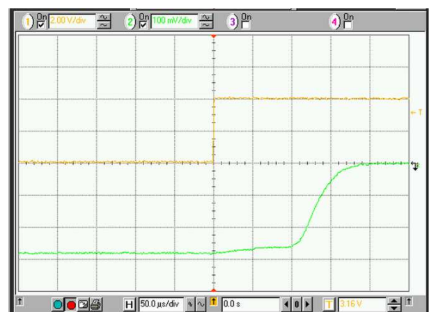
Switching time RF On (TTL 0) to RF Off (TTL 1) (Yellow - TTL, Green - RF signal)
