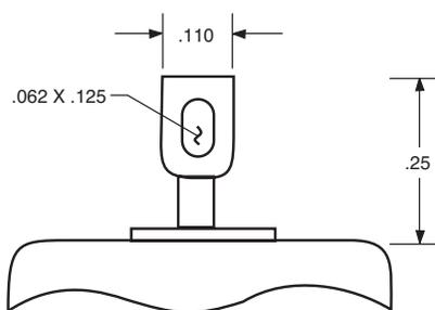
Figure 2. Optional Loop Type Solder Terminal
