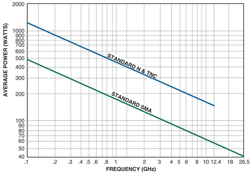
**Power Handling Capability of Narda Switches vs. Frequency for Common RF Connectors**
