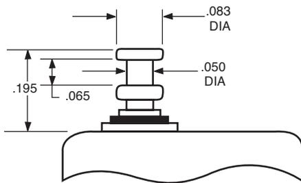
Figure 1. Standard Solder Terminal
