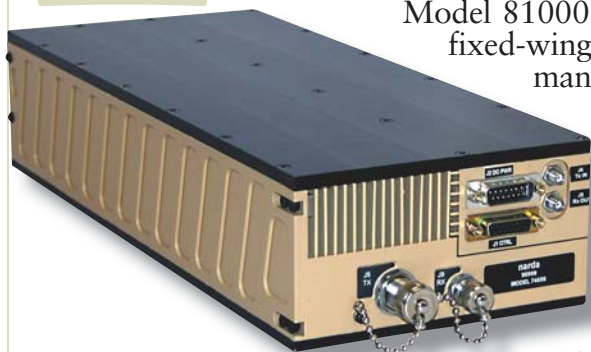
1. Model 81000 is a satcom transceiver mounted in a rugged enclosure measuring 15 x 6.25 x 3.25 in., and weighing a manageable 15 lb.
